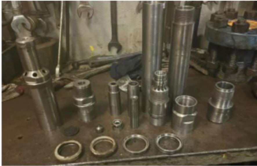
CONVENTIONAL JET PUMP 3-1/2"x2.81" INSPECTED AFTER LIFTING JOB
