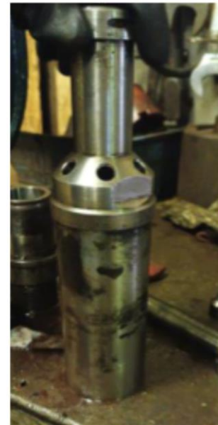
FISHING NECK PRESENTS STAINS CAUSED BY POWER FLUID. THE FISHING NECK IS FOUND WITH A CONSIDERABLE AMOUNT OF SEDIMENTS AND SCALE OBSTRUCTING THE POWER FLUID ENTRANCE
