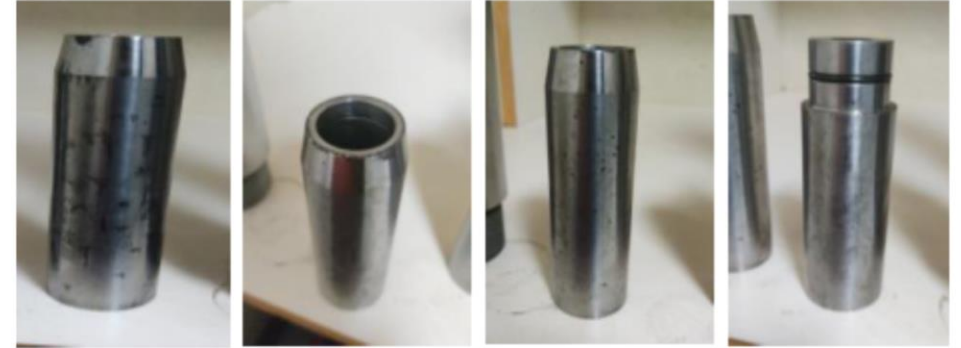
JET PUMP RECOVERED WITH OPERATIONAL NOZZLE AND THROAT WITH NORMAL WEAR. UPPER AND LOWER TEFLON SEALS WITH WEAR AND SCRATCHES. HOUSING THROAT WITH STINGS AND SCRATCHES (WEAR IS PRESUMED DUE TO METAL SOLID PRESENCE DURING OPERATION). OPERATIONAL DIFFUSER.
