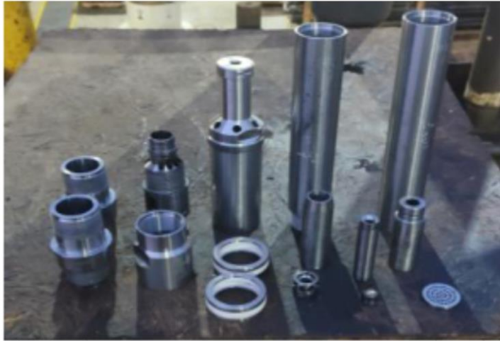
JET PUMP DISASSEMBLY. ALL PARTS IN GOOD CONDITION.
