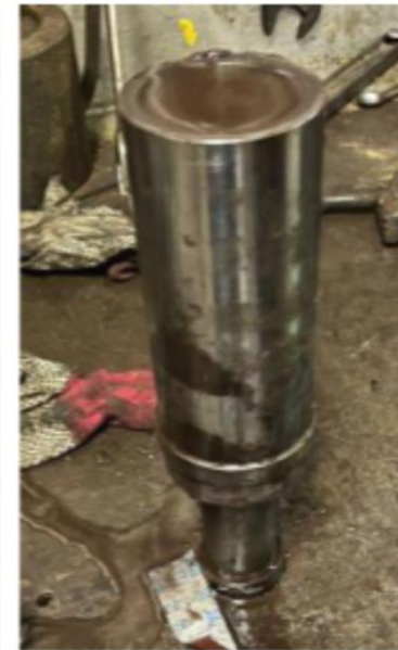
FISHING NECK PRESENTS STAINS CAUSED BY POWER FLUID. THE FISHING NECK IS FOUND WITH A CONSIDERABLE AMOUNT OF SEDIMENTS AND SCALE OBSTRUCTING THE POWER FLUID ENTRANCE
