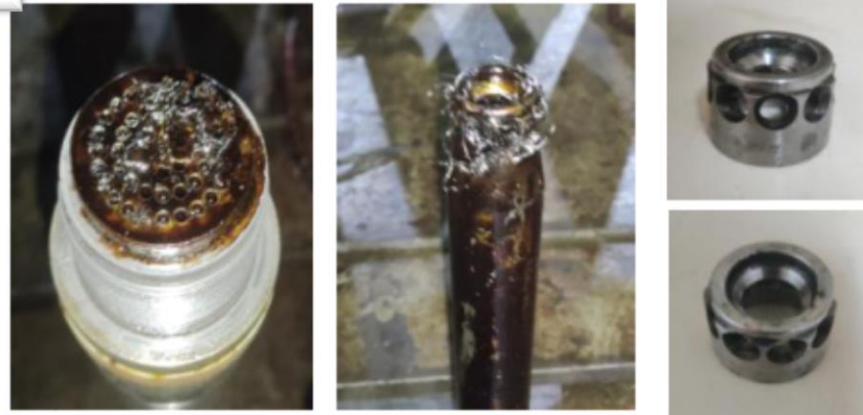
FILTER PLUGGED 30% DUE TO SEDIMENTS AND SLAG, NOZZLE RETAINER WITH METAL FIBERS (PRESENTS WEAR), OPERATIONAL DIFFUSER.
