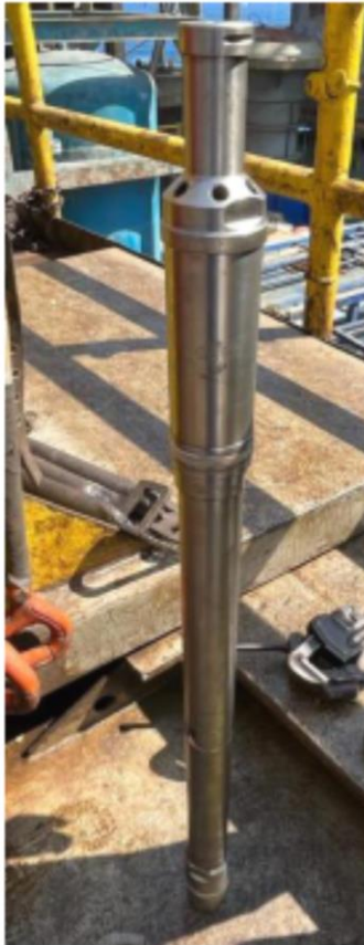
JET PUMP SET TO RIH
